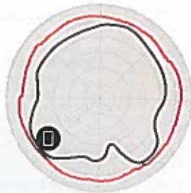
Figure 2 - T310d 2.4GHz Azimuth Antenna Patterns
