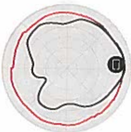
Figure 3 - T310d 5GHz Azimuth Antenna Patterns
